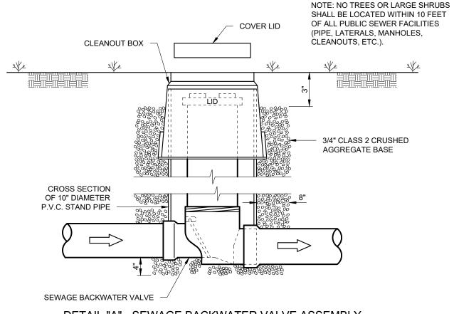
DETAIL "A" - SEWAGE BACKWATER VALVE ASSEMBLY
