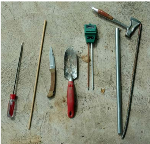
All these instruments can be used to gauge soil moisture: a long screwdriver, wooden dowel, knife, hand trowel, moisture meter, and a thin-walled pipe, hammer and rebar.
